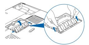
Figure 4-13. Removing a Memory Upgrade Module
